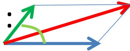
$$F_1 = 100 \quad F_2 = 60 \text{ (N)} \quad F = \dots ?$$
